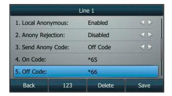
6. Press the **Save** soft key to accept the change or the **Back** soft key to cancel. Anonymous call is configurable via web user interface at the path **Account->Basic.**
